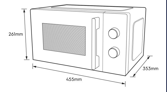
Please note! Dimensions to be used as a guide only. All customers MUST refer to the user manual supplied with the product for detailed installation instructions. © 2021 Electrolux S.E.A PTE. LTD. E\_DIM\_EMM20K22B\_TW\_Oct21
