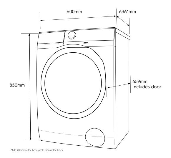
Please note! Dimensions to be used as a guide only. All customers MUST refer to the user manual supplied with the product for detailed installation instructions. © 2021 Electrolux S.E.A PTE. LTD. E\_DIM\_EWF1141R9SB\_Jun21
