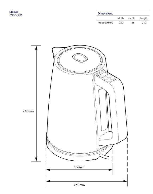
Please note! Dimensions to be used as a guide only. All customers MUST refer to the user manual supplied with the product for detailed installation instructions. © 2022 Electrolux S.E.A PTE. LTD. E\_DIM\_E5EK1-51ST\_Jun22
