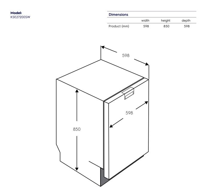
Please note! Dimensions to be used as a guide only. All customers MUST refer to the user manual supplied with the product for detailed installation instructions. © 2021 Electrolux S.E.A PTE. LTD. E\_DIM\_KSE27200SW\_Jun21
