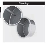
1.Turn the machine off and let it cool down. Wipe all outer surfaces with a damp cloth. Clean clogged holes in the filter and filter holder with a pin or small brush.
